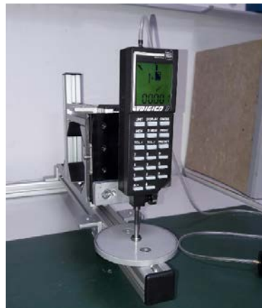
Set-up for testing fabrics (pool swimsuits) Pressure 1 +/- 0.01 kPa
