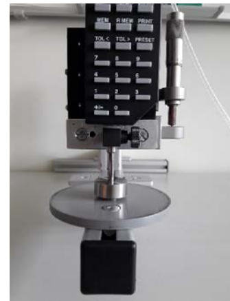
Set-up for testing insulating material (wetsuits) Pressure 10 +/- 2 kPa
